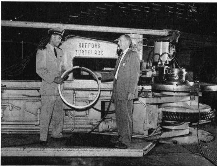
From left to right, the Turnblades—Ensign Richard Turnblade, Delta Delta '53, U. S. Navy, the Hufford Turnblade stretch-wrap forming machine, and Charles Turnblade, father of the Naval officer and designer of the unusual machine which bears his name. The photo was taken at Douglas Aircraft's El Segundo (Cal.) Division, where Ensign Turnblade formerly worked in the engineering department. During a recent leave, Ensign Turnblade visited the company to see his father, and took the opportunity to see the versatile machine which can form 360° parts
